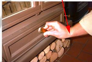
To adjust ash pan door handle, open the drawer, wind the handle clockwise until it stops. Push drawer against stove body, then unwind handle anticlockwise until it locks into place. It should now only need a quarter of a turn to open or close drawer
