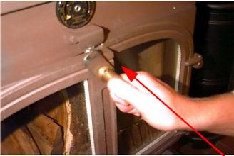
Door handles are adjustable for tension. To make adjustments open door and turn handle anti clockwise for one turn. To loosen catch turn handle clockwise
